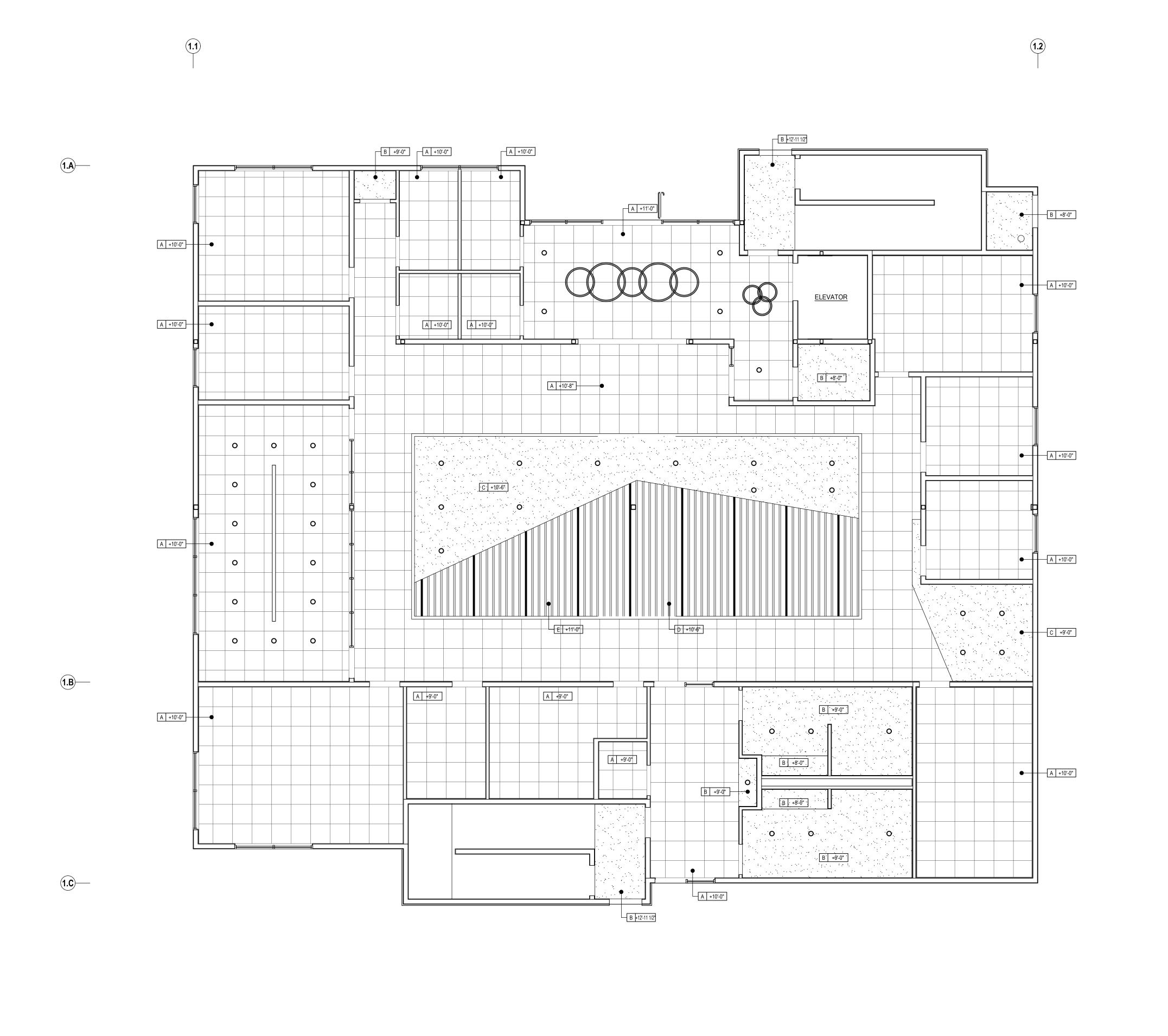
CEILING FINISH TYPES A = 2'x?' SUSPENDED CEILING SYSTEM-? B = GYPSUM BOARD TAPED, TEXTURED & PAINTED ON CEILING JOISTS PER PLAN. C = ARMSTRONG SUSPENDED DRYWALL GRID SYSTEM w/ GYPSUM BOARD TAPED, TEXTURED AND PAINTED. D = LINEAR ACOUSTICAL BAFFLES E = NO CEILING. (OPEN TO FRAMING) NOTE: SEE SHEET A3.2 FOR SUSPENDED CEILING DETAILS
